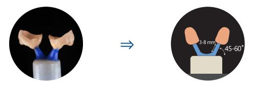
Connect the object and investment ring base at an ∠45~60° angle, at a length of 3~8mm, using Ø3~3.5 mm of spruing wax.
