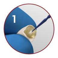
After try-in, etch the inner surface with 5% hydroflouric for 20 seconds.
